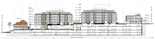
Figure 1 – Section through the whole block between Victoria Avenue and Albert Avenue - looking East, showing that the changes subject to this application (bubbled shown on top of buildings) are mainly limited to lift over run and clerestory
